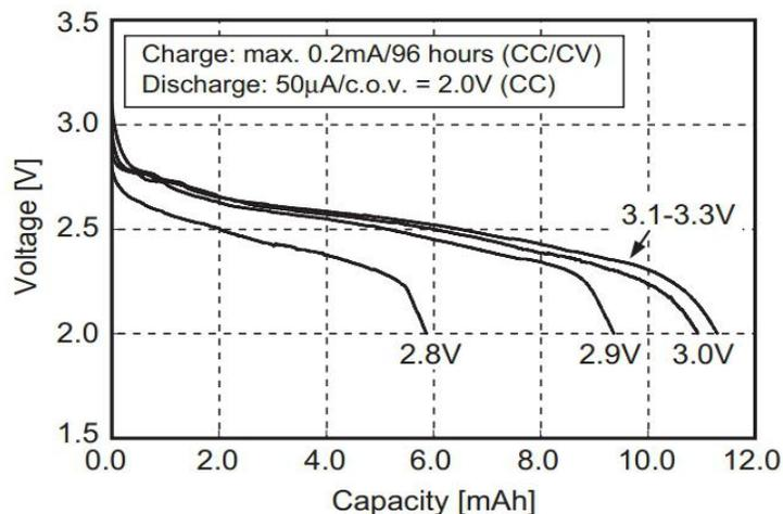
**Figure 7:** Seiko MS920SE Charge and Discharge Characteristics
