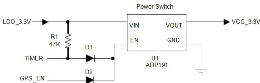
**Figure 6:** The External Switch Circuit for TIMER
