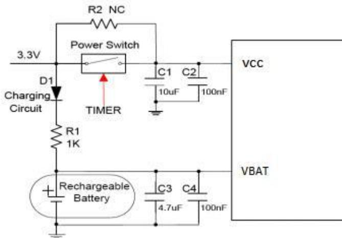
**Figure 5:** Reference Charging Circuit for Chargeable Battery
