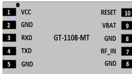
**Figure 2:** Pin Assignment
