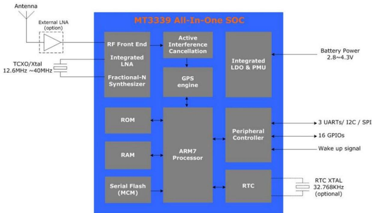
**Figure 1:** Block Diagram
