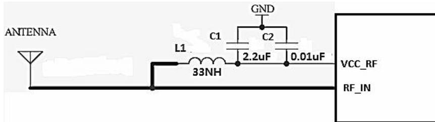
**Figure 14:** Reference Design for Active Antenna
